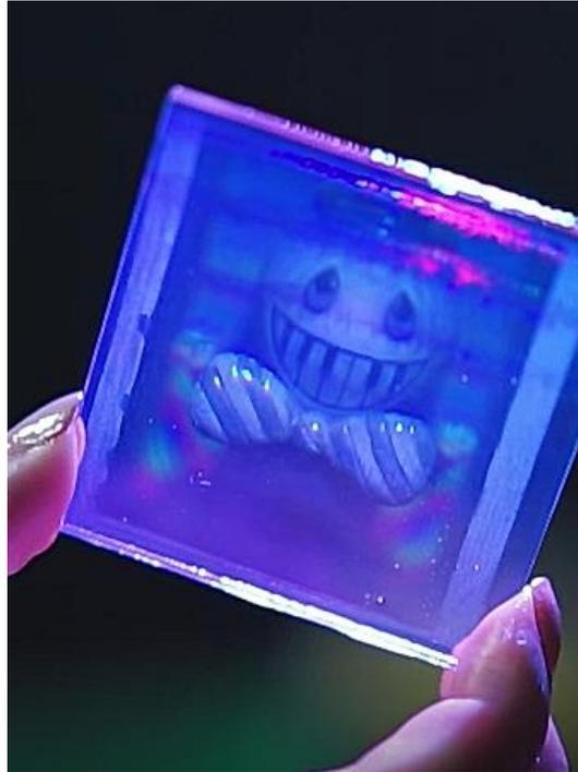
*Hologram observed by transmission via halogen spot, after bleach.
